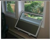
Lower the top sash three to four inches above the bottom sash. Using the tilt release latches at the top corners of the sash, push them towards the center of the sash and tilt the sash inward and allow it to rest on the bottom sash. This will allow you to clean and it will not become disengaged from the pivot shoe. Holding the sash horizontally or parallel to the floor can allow the sash to come out of its pivot shoe while cleaning.
